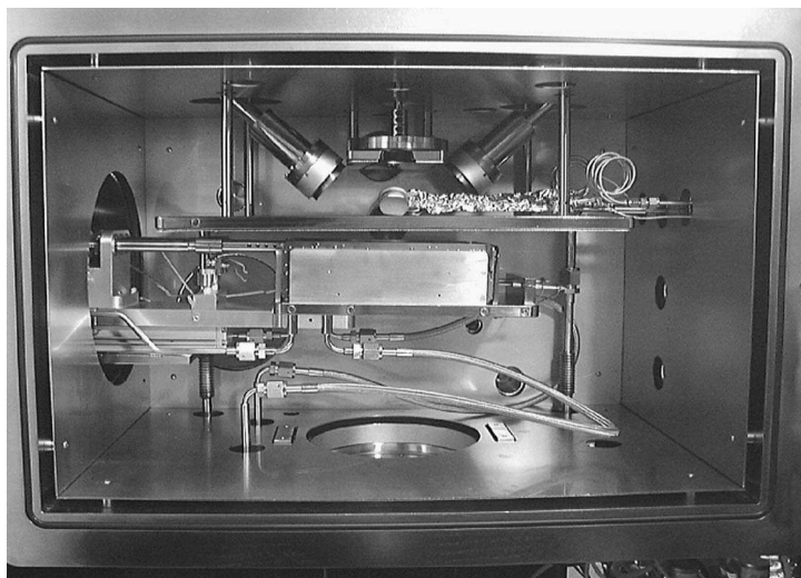
Figure 23.1 Large deposition chamber for pulsed laser ablation and magnetron sputter depositing hybrid. Laser ablation target is in the upper center of the chamber and two magnetron sputter guns are at the chamber upper left and right.
