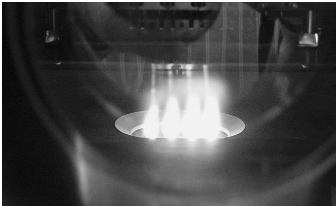
Figure 9.17 Photograph of a multiplume system. Seen clearly are four plumes coming through the large cutout in the water-cooled plate that sits directly above the large target surface.
